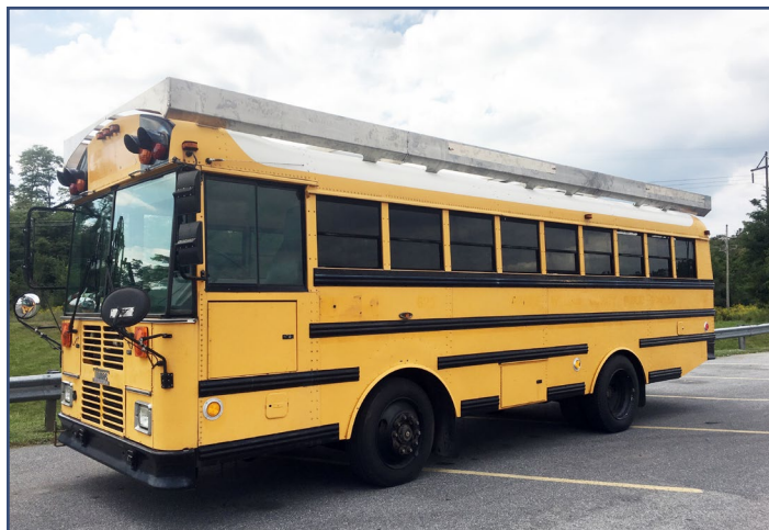
Completed solar rack installed on the bus.
