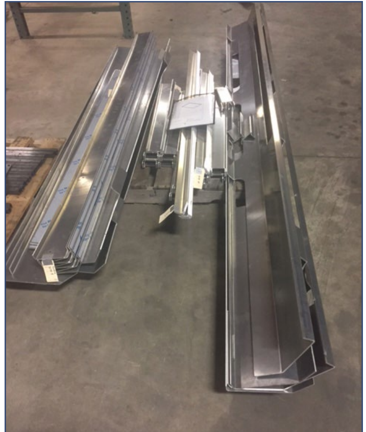
Precision-cut solar rack pieces, awaiting seamless fabrication.
